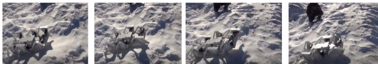
Figure 2.20: Outdoor test of the water resistant BigAnt on the wave field that is covered by 10+ cm depth of snow.
