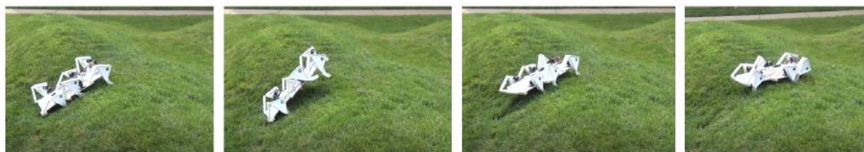
Figure 2.19: BigAnt outdoor tests on the grass wave field.
