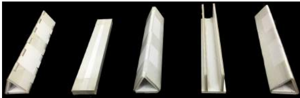
Fig. 6. Structural members made using PARF techniques. [left to right] Notched prism, layered plates, cut-folded prism, hot-glued fins, and crush-folded prism. Each was made from a 30.5 cm \times 15 cm piece of foam board.
