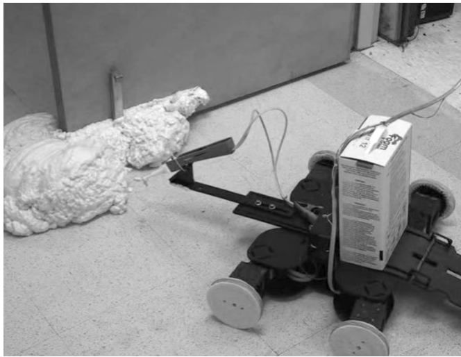
Fig. 7. Foam synthesizer pours a doorstep that firmly locks a door in place
